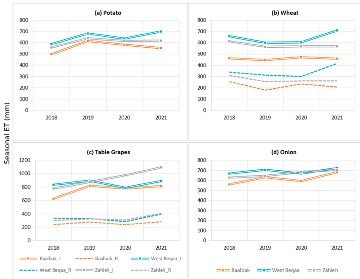
Fig. 6. Mean seasonal actual ET estimates of potato (a), wheat (b), table grapes (c), and onion (d) over four years (2018–2021) of WaPOR V2 water use data components distinguished by district in the Upper Litani Basin (I = irrigated; R = rain-fed).
